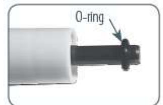
Reassemble the pipette. Depending on the pipette model the dimension of the O-ring will vary (refer to chapter 19).
